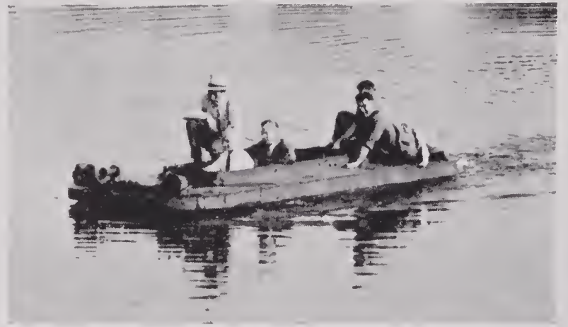
FIGURE 35. In water, pilot model of T-15 Weasel remains afloat but tracks give little net horizontal thrust or steering control.
